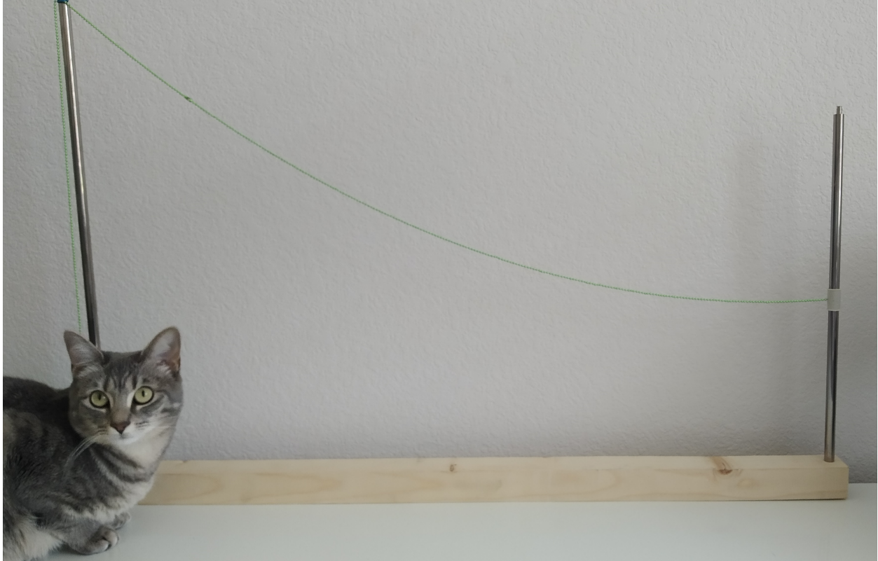
Figure 8: If one of the ends can freely slide, it will settle down to the point for which the chain leaves from the shaft at an angle of 90^\circ . The curious cat is for scale.
