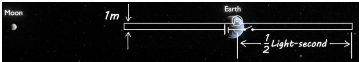
Figure 8: A circuit that extends halfway to the moon. The load is only 1m away from the battery. Image taken from Veritasium video.
