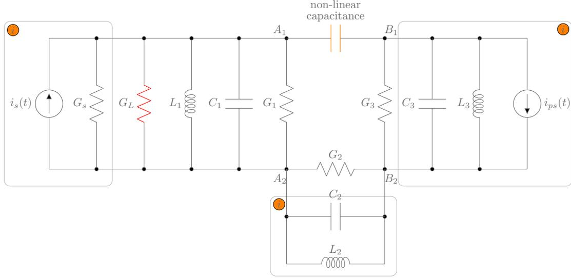
Figure 1: Non-degenerate parametric amplifier[2]. Hover over the orange circuit elements to see more information.
